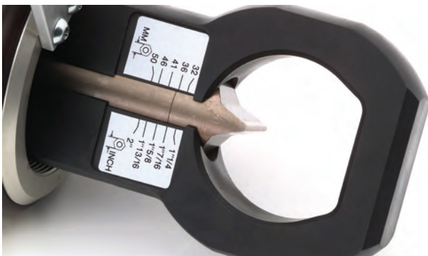
Adjustable blade; prevents damage to the thread
